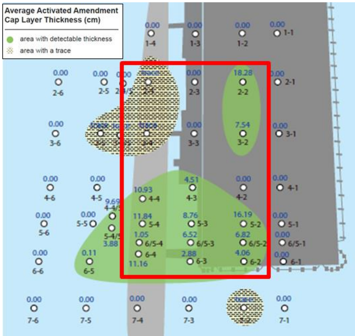
Figure 13. Comparison of intended cap target area with the actual cap presence measured in the August 2013 (10-month) SPI survey.
