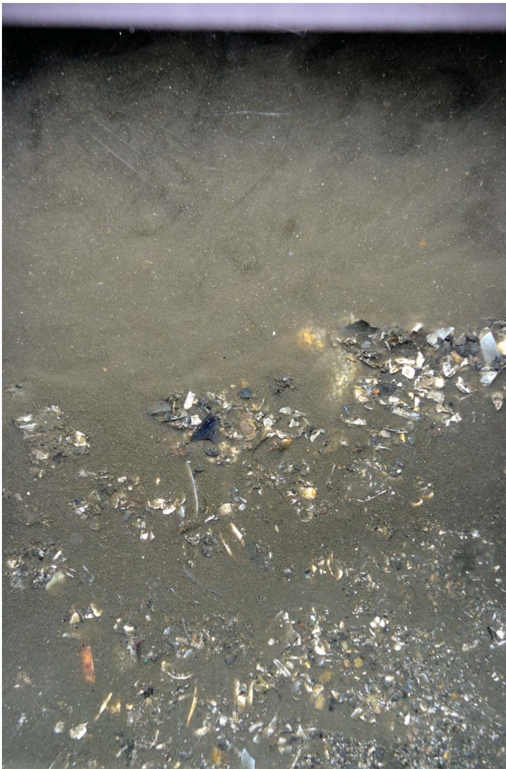
Figure 12: This profile image from Station 1-3 is typical of many of the images collected by divers and shows the lack of preservation of any subsurface features due to the prism being wiggled to insert it in the sediment. Scale: width of image = 14.5 cm.
