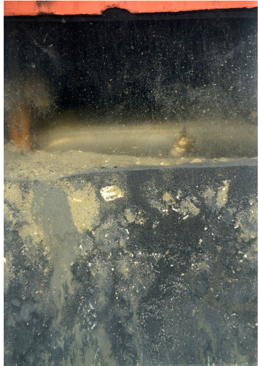
Figure 17: These profile images from 2012 and 2013 at Station 6-4 show the small-scale heterogeneity in the spatial distribution of the reactive amendment added in Oct 2012. Scale: width of each image = 14.6 cm.
