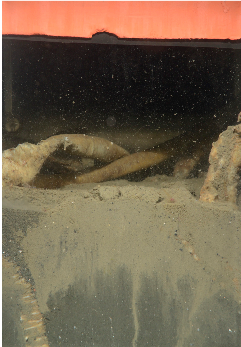
Figure 17: These profile images from 2012 and 2013 at Station 6-4 show the small-scale heterogeneity in the spatial distribution of the reactive amendment added in Oct 2012. Scale: width of each image = 14.6 cm.
