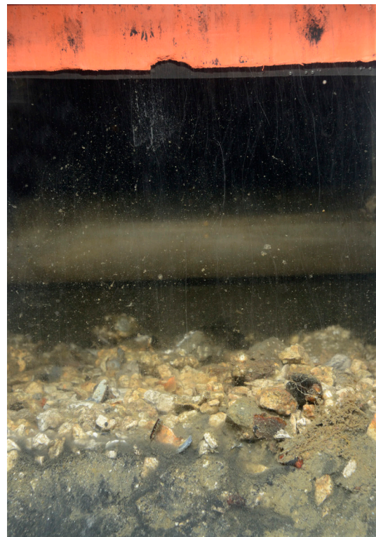
Figure 8: These profile images from the same stations taken in 2012 and 2013 show the radical change in sediment type because of the appearance of the surface armoring of cobble and shell; compare the differences in images from Station 1-3 (top) and 4-3 (bottom). Scale: width of each profile image = 14.6 cm.
