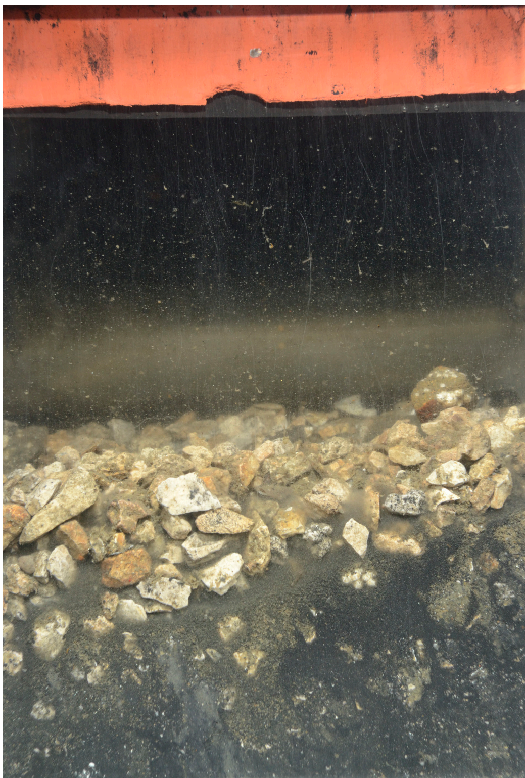
Figure 10: This profile image from Station 5-3 shows a distinct layer of the white pebbles that were coated with the reactive amendment and used as a carrier to get the material to the bottom sediments; particles of activated carbon are still visible in the subsurface profile. Scale: width of profile image = 14.6 cm.
