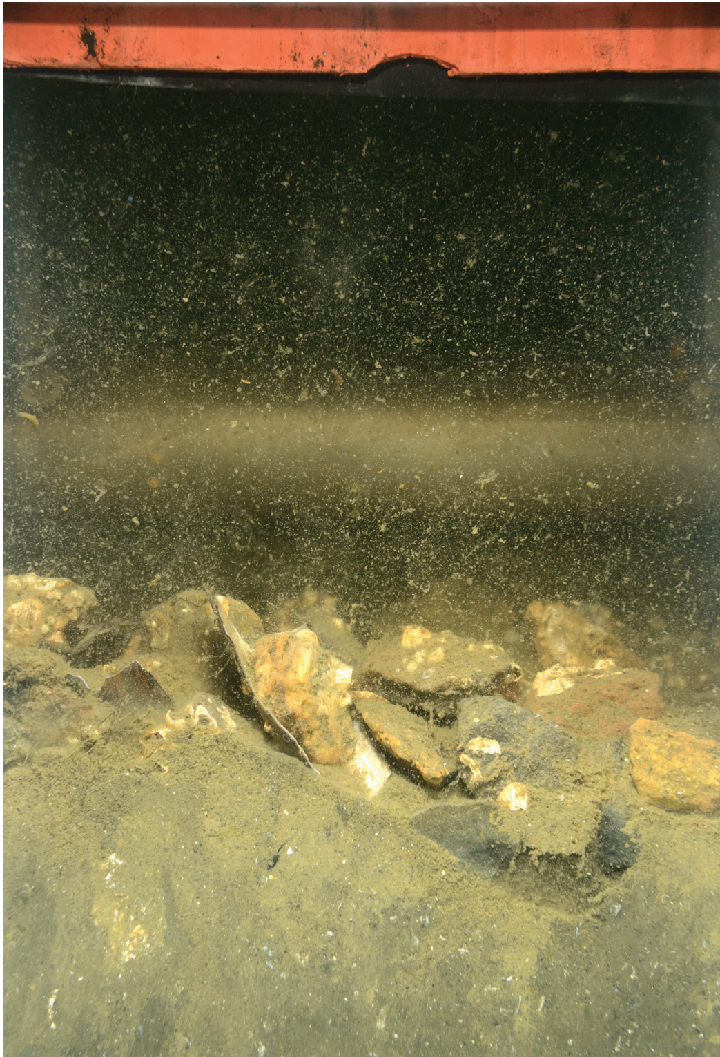
Figure 6: As in past surveys, the SPI photos from Station 1-3 show an armoring of pebble and cobbles over silty very fine sand. Scale: width of profile image = 14.5 cm.
